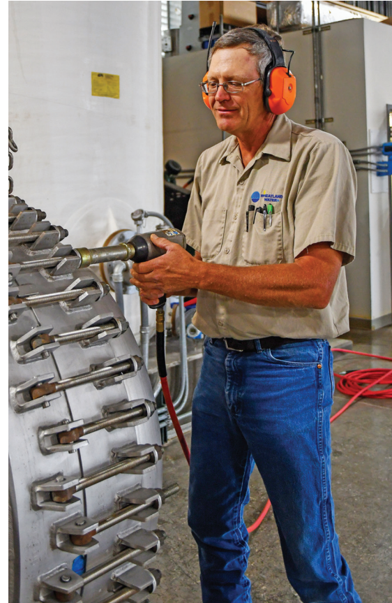
Francis Lobmeyer removes the retaining bolts from a cartridge filter that houses the micron disposable filters. There are 42 bolts to remove on each housing which are removed with an impact tool. This is a labor intensive and expensive job to complete.
